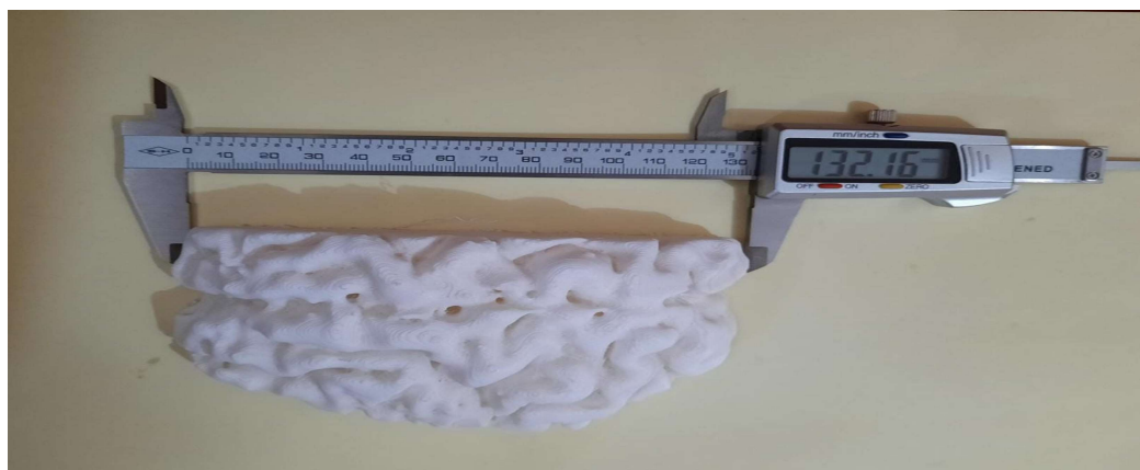
Figure.2 The distance measured from anterior to posterior (AP) using a digital caliper.
